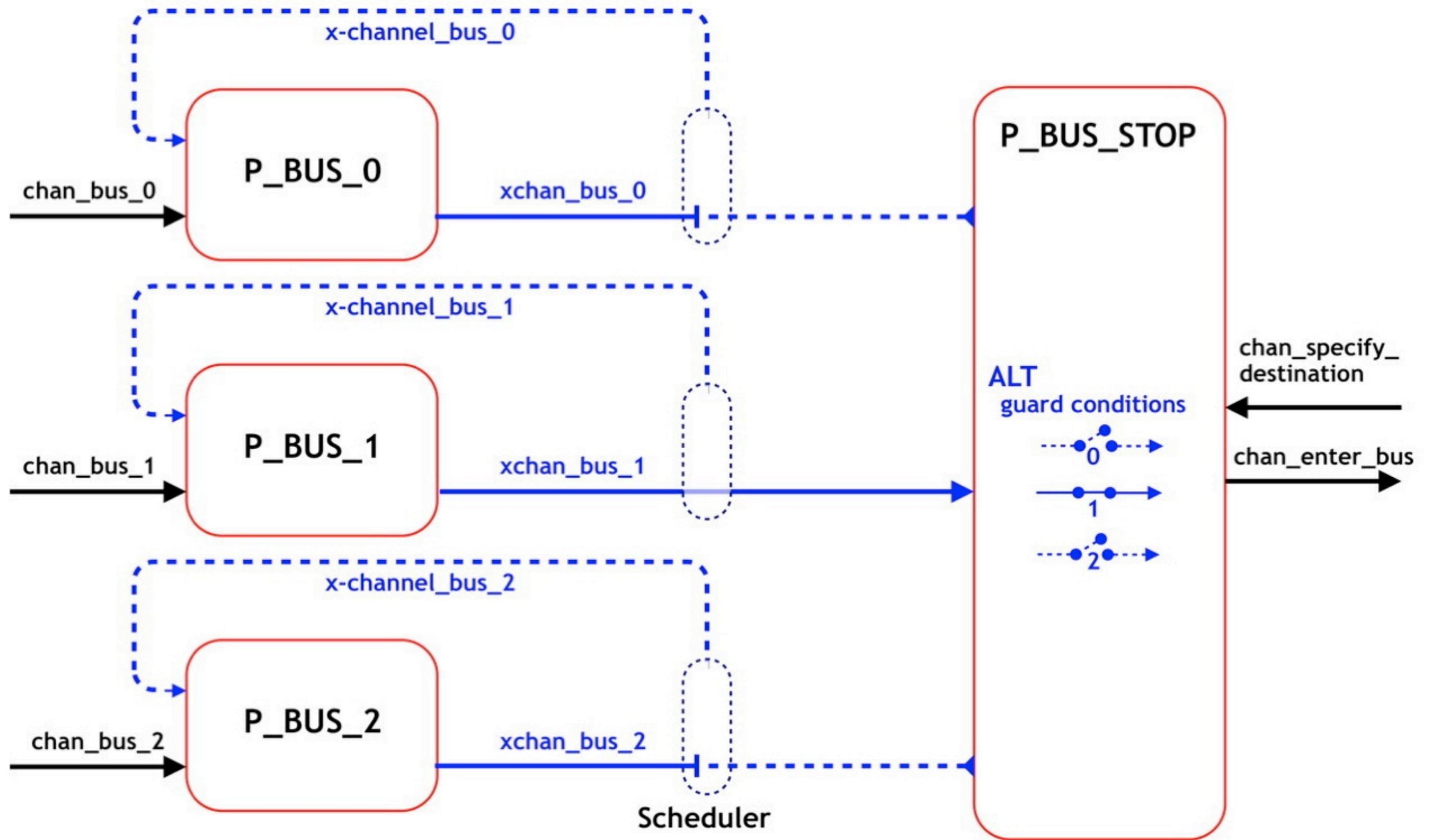
Figure 2. XCHAN (array of 3) and feathering, with only bus #1 as possible to ride
